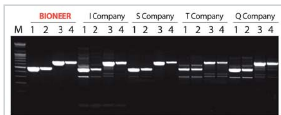
Figure 1. Comparison of PCR amplification specificity between AccuPower ® PyroHotStart Taq PCR PreMix from Bioneer and other suppliers' HotStart PCR Master Mix. PCR reactions were performed according to each supplier's protocol. The PrP gene was amplified from human genomic DNA with two different primer sets, separately. This data shows that AccuPower ® PyroHotStart Taq PCR PreMix has higher amplification efficiency and specificity than other suppliers' HotStart PCR Master Mixes.
