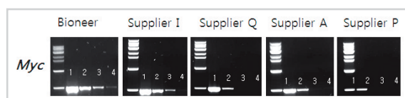
Figure 4. Comparison of amplification results between Bioneer AccuPower® RocketScript™ Cycle RT PreMix and suppliers' RTases
